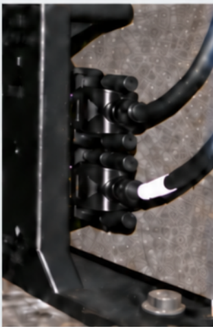
LTC 3D printed bracket installed on USMC vehicle (representative example).
